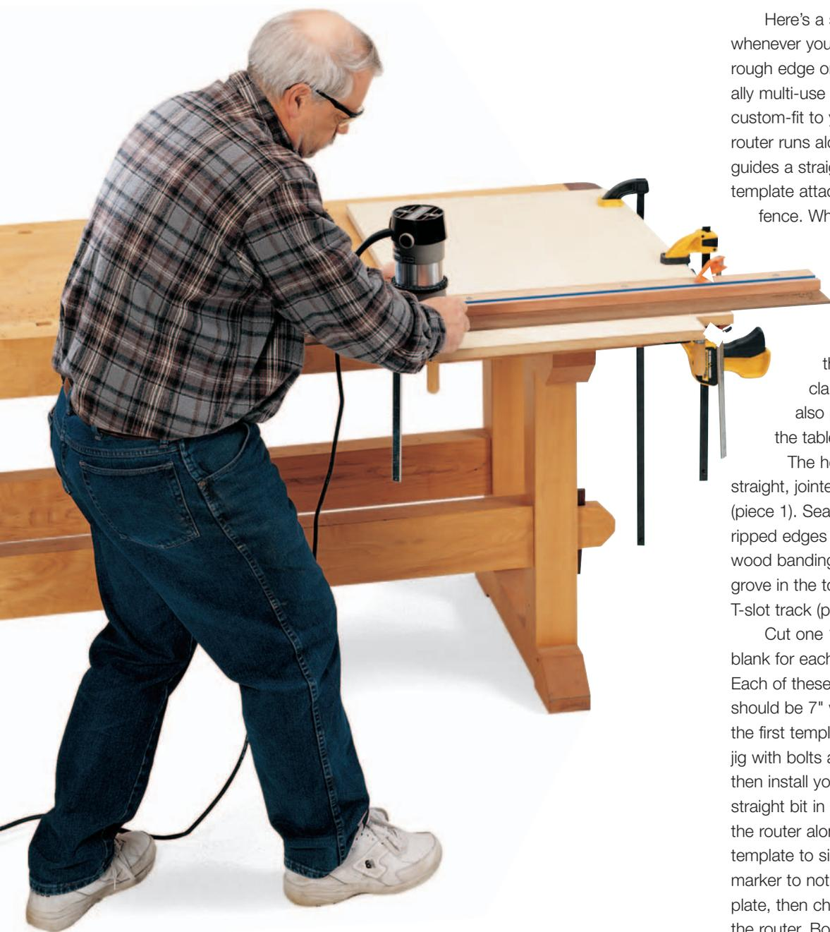
Here's a slick jig to have handy whenever you need to straighten a rough edge or plow a groove. It's actually multi-use straightedge, designed to custom-fit to your portable router. The router runs along its fence, and that guides a straight bit along a hardboard template attached to the bottom of the fence. Whenever you need to make
