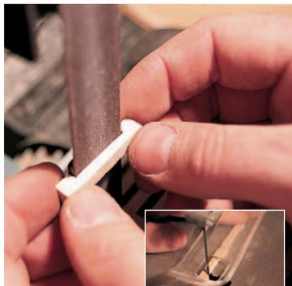
**Step 5:** The moving jaw is locked in its travel along the bar (piece 3) by a pair of maple wedges (pieces 4). Scroll saw these wedges to rough shape, (see pattern at left) and use a small belt sander or a file to refine the cut. Be sure you don't over-sand the wedges or they'll lose their locking action. This has to be a tight fit.
