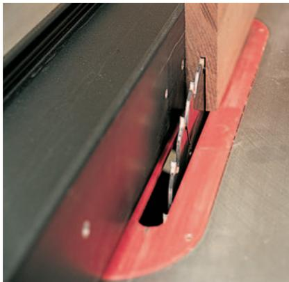
**Step 1:** Rip hardwood scraps to 3/8" thickness to make the jaw halves (pieces 1 and 2). Tight-grained hardwoods such as maple and walnut work best, but any strong, straight stock will do. For safety reasons, rip halfway through a wider piece for your first cut (as shown above), and then lay the piece flat to cut it to width.
