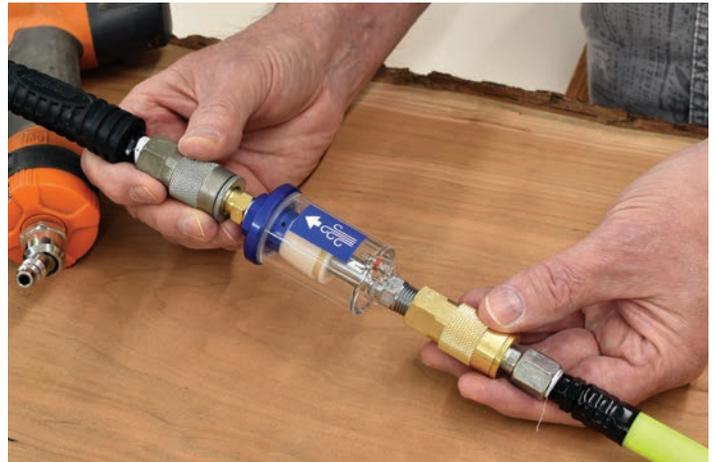
**To keep liquids from entering tools, an inline filter – installed between the compressor and tool – helps minimize the amount of water traveling through the hose.**
