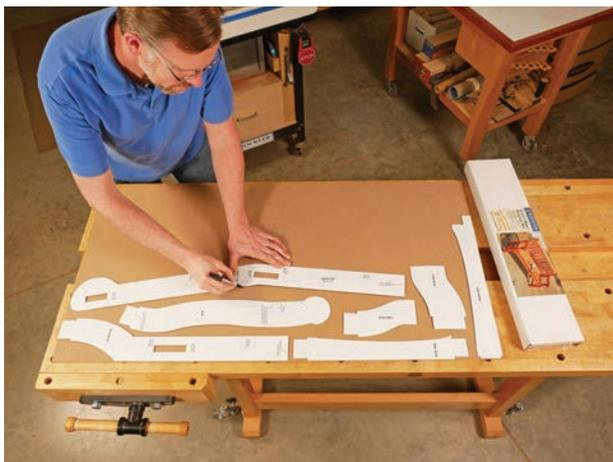
You can create full-size tracing patterns by enlarging the gridded drawings on the second page of this PDF. Rockler also offers a kit (shown above) containing all the cardboard patterns you'll need to build this bench project. Either way, full-size patterns are an essential part of the building process.
