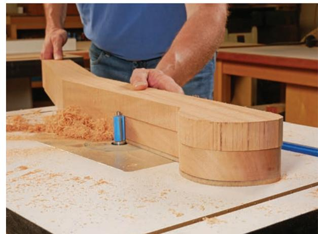
Rigid templates will help you reproduce this bench's curved and angled shapes at the router table. Here, the template is mounted to the bottom of this bench leg workpiece as it's being template-routed to final shape. Make your templates from 1/4" hardboard, plywood or MDF, using your full-size patterns to trace the template shapes.
